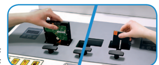
Separate feed openings for 3.5" and 2.5" drives
