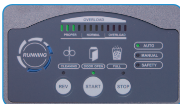
Control Panel includes LED load indicator, safety key and emergency stop button
